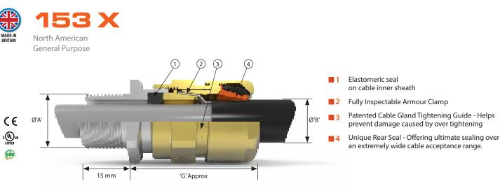
The 153/X Cable Gland is general purpose cable gland for use with wire braid, steel wire armour, elastomer and plastic insulated cables. The gland provides an elastomeric seal on the cable inner sheath, and a low smoke, zero halogen IP and retention seal onto the cable outer sheath.
