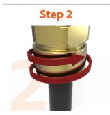
Tighten backnut until a seal is formed onto the cable, then tighten one further turn
